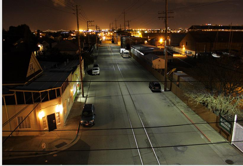
Yellow HPS “hot spots” on the road are replaced with uniform white light. Energy savings up to 70%.
