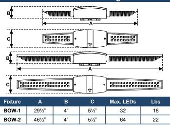
The new Bow LED luminaire from Visionaire, simplifies the task of selecting the best solution for LED parking garage lighting. The linear design of the luminaire, compliments the linear design of the pre-cast concrete coffers; creating an integrated lighting effect; and maximizes the perceived lighting coverage. It is an ideal replacement for the high-maintenance fluorescent fixtures of yesterday.
