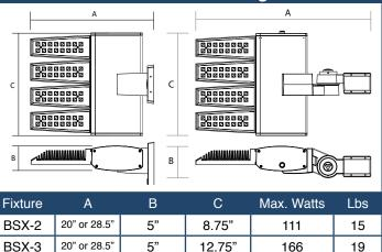
The new BOW SX LED Series continues the unique contemporary design inspired by the sleek styling of the BOW family. Separating the extruded aluminum driver housing and the individual die-cast aluminum linear LED engines: optimize the life of the LEDs and the Driver(s); and maximizes the lumen output of the fixture.
