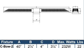
The Cross Bow LED Series continues the unique contemporary design inspired by the sleek styling of the Bow<sup>TM</sup> family. Separating the Driver(s) from the individual die-cast aluminum linear LED engines: optimize the life of the LEDs and the Driver(s); and maximizes the lumen output of the fixture.
