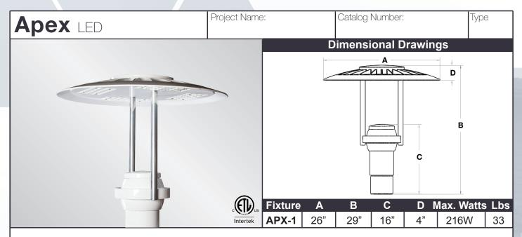
The new Apex LED Series offers clean, functional styling that blends with a broad range of architecture. The cast aluminum housing with integrated pole top fitter anchors aluminum mounting rods to support the cast aluminum shade that houses the LED light engine. The LED's performance and the driver's life are maximized by enclosing them in the two separate compartments.
